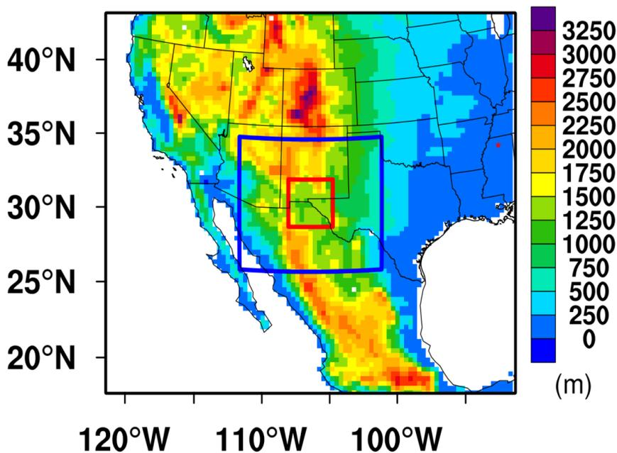
Figure 2.1 Configuration for the concentric nested CAMx domains (The three domains are in 36-, 12- and 4-km horizontal resolutions. Shaded contours are terrain height with unit of meters)
