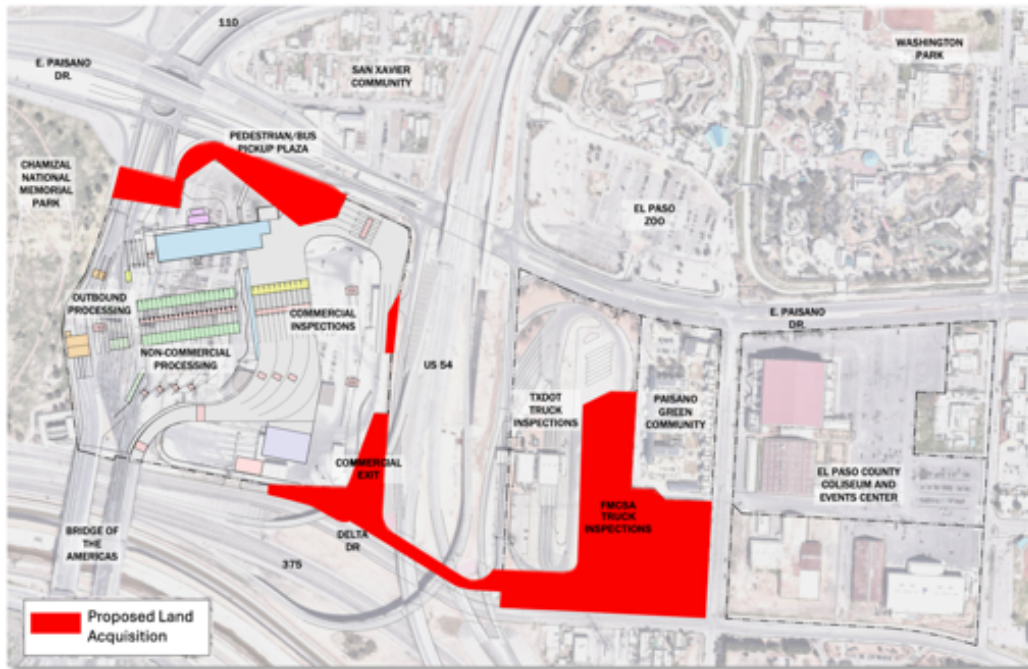
Figure ES-1. Viable Action Alternative 1a General Site Design/Layout and Land Acquisition.
